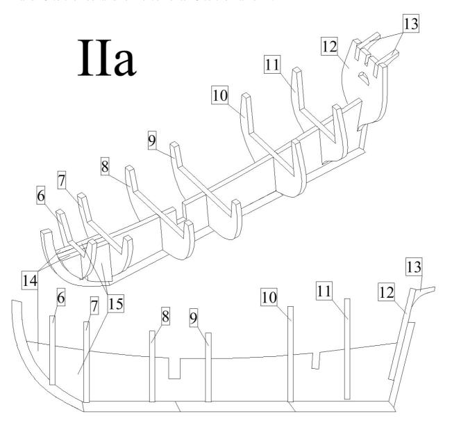
b) First run a deck 16 to the frames and then glue all frames, deck and keel together.
