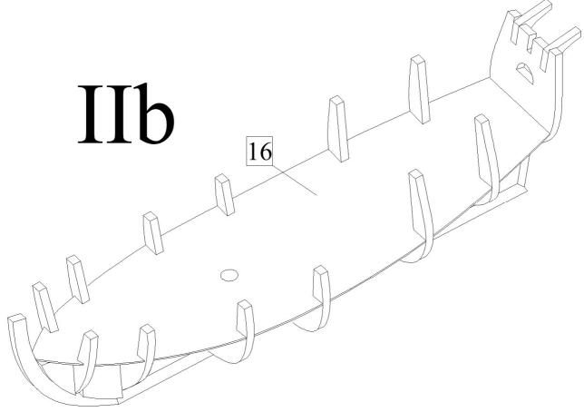
c) Sharpen frames and reinforcement as it is shown below.
