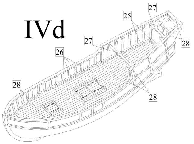
e) First glue a deck 29 to the transverse beams 27. Then plank the deck by strips 30 and then edge it by strips 31.
