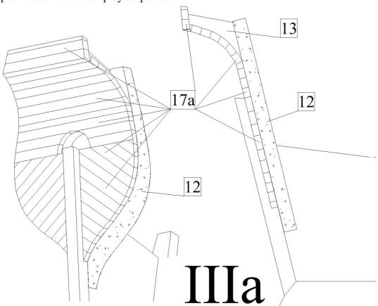
b) Plank a hull of the ship by strips 17b. Before planking bend the strips into required shape (A procedure of the strip bending is described in a start of this document). Start the planking from stem with strips on upper edge of the hull. Then continue with planking to the stern.
