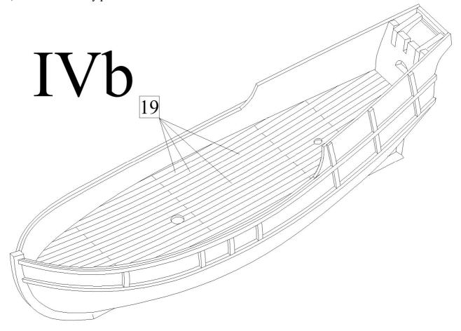
c) Make hatches on the deck. First glue frames of the hatches from parts 20, 129 and 130. Then glue this frames to the deck. Then plank the hatches by strips 21. Finally glue parts 22-24 to the hatches. The hatches are in 1:1 scale shown in the plan 4.
