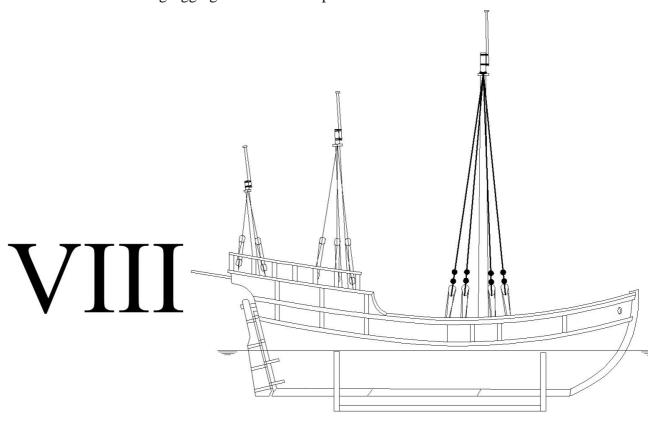
a) First glue masts 64-66 to the hull. Then tie shrouds 50 to the mast 64 and shrouds 49 to the masts 65 and 66. Tie violin blocks 115 to the end of the shrouds 50 and block 72 to the shrouds 49. Then tie the shrouds by a rope 49 to the eyebolts. A scheme of tying of the shrouds is shown in the figure below.
